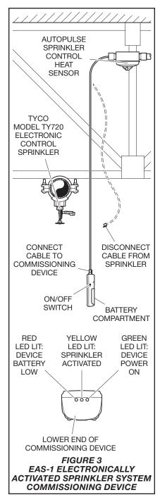
lated sprinkler operation for a typical system. If the system is designed to operate a maximum of nine sprinklers, only nine out of the 10 Commissioning Devices should be observed with a Yellow LED lit indicating sprinkler operation.
