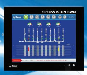
SPECSVISION-BWM is a useful tool for predicting bearing wear in 2-stroke engine before it becomes critical condition and the system provides early alarm or slowdown signal if unexpected problem occurs at the crank-train bearings comprised of crosshead, crank and main bearings during engine operation.
