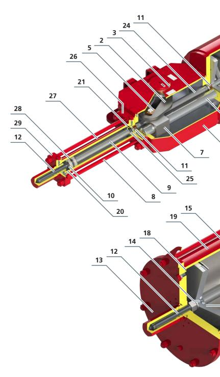
For quarter-turn pneumatic applications with torque requirements below that of the GP range, Rotork Fluid Systems offers two smaller ranges of scotch yoke actuators with outputs up to 4,500 Nm (39,828 lbf.in). Consult PUB013-001 (CP range) and PUB014-001 (RC200/RCI200 range).
