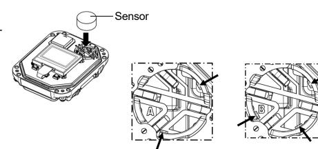
Locations to match when fitting the sensor (CO-04/HS-04/SC-04 (SO2))
