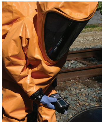
CBRN detection with the MultiRAE Pro
