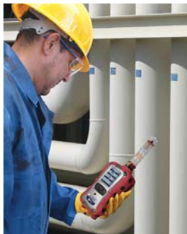
Multi RAE Benzene used for leak detection
