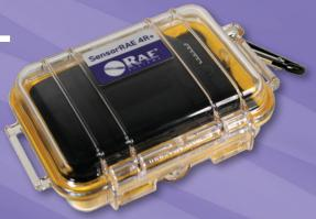
The compact, waterproof SensorRAE 4R+ sensor conditioning station keeps up to six extra sensors warmed up and ready for quick deployment in MultiRAE or ToxiRAE Pro monitors. The SensorRAE 4R+ keeps spare sensors on bias and readily available for use¹ without the extra warm-up time after installation required by sensors such as ethylene oxide or nitric oxide.
