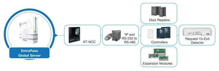
\*Note - IP requires UDS1100 serial Ethernet converter for Ethernet connection to the controller
