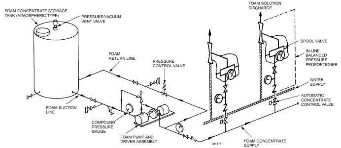
NOTE: Flush connections are only required with protein based foam concentrates.
