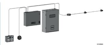
Green, amber, and/or red pulsing LEDs and the internal sounder alerts at the display for real-time system status. The sounder only activates for alarm, trouble, or supervisory signals.
