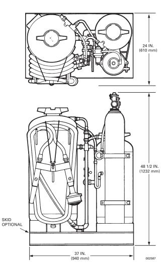
The AFFF can be used to secure unignited spills as well as suppress and secure spill fires which cannot be accomplished with dry chemical alone. When used in combination, three dimension, running and pressure fires can be suppressed by a single trained operator.
