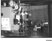
The Mini-Bulk Low Pressure CO<sub>2</sub> Fire Suppression System is designed to meet the requirements of NFPA 12, "Standard on Carbon Dioxide Extinguishing Systems." The system consists of a low pressure storage tank, discharge valves, manual and automatic controls, distribution nozzles, alarms, indicators, and supervisory devices as required to maintain a supply of carbon dioxide in a discharge-ready state, and to provide effective distribution of agent on demand.
