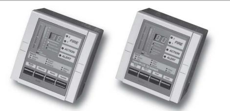
Display modules provide real-time indication of the status of an Xtralis VESDA detector. They have a 20-segment vertical bar graph display, a 2 digit numeric display, an audible sounder, clear alarm and fault indicators. They also have 4 push button keys to control the detector and the mode of the display.
