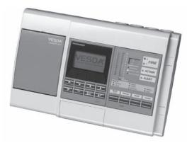
The Xtralis VESDA VLP detector is the central element of the Xtralis VESDA ASD product range. Using unique detection principles, the VLP has an alarm sensitivity range of 0.0015%–6.25% obscuration/ft (0.005%–20% obscuration/m). The VLP is classed as a "Very Early Warning Smoke Detector". This means that it detects fire at the earliest possible stage and reliably measures very low to extremely high concentrations of smoke.
