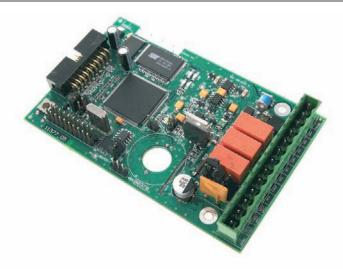
The Xtralis VESDA VLF MCC (Multi-function Control Card) is an interface card for the range of Xtralis VESDA VLF smoke detectors. An MCC expands the range of input and output communications a VLF can perform.
